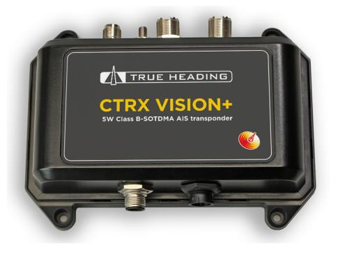
The new True Heading CTRX Vision+ is a modern 5 Watt AIS class B transponder, which uses the SOTDMA protocol. Just like AIS class A equipment, CTRX Vision+ participates in the time slot reservation plan, so it will always have a free timeslot available to transmit it's position, at a higher update rate.
